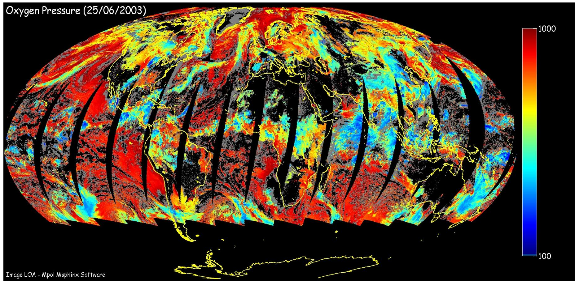
Differential absorption is used to infer cloud top (middle) pressure - 763nm and 765 nm
